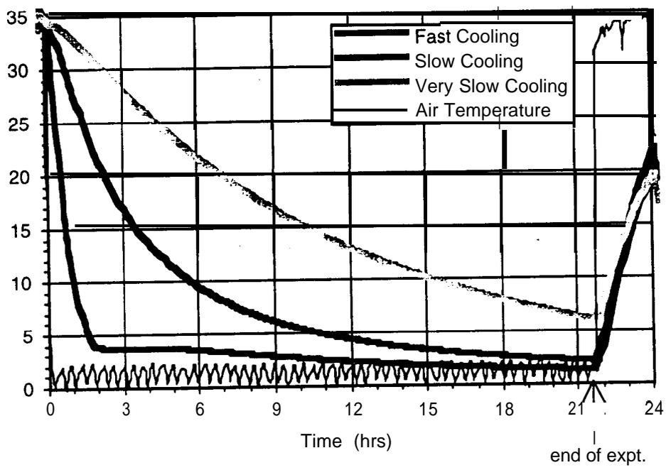
Figure 1. Example of cooling times for the three cooling treatments.
